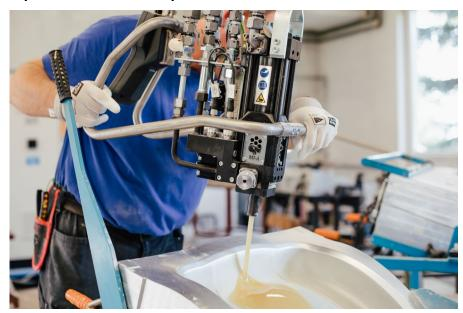
The HIGHLINE MK2 in use at PKS: manual production of even the smallest series in premium quality – even under difficult conditions such as demanding part geometries or special fire protection requirements.
