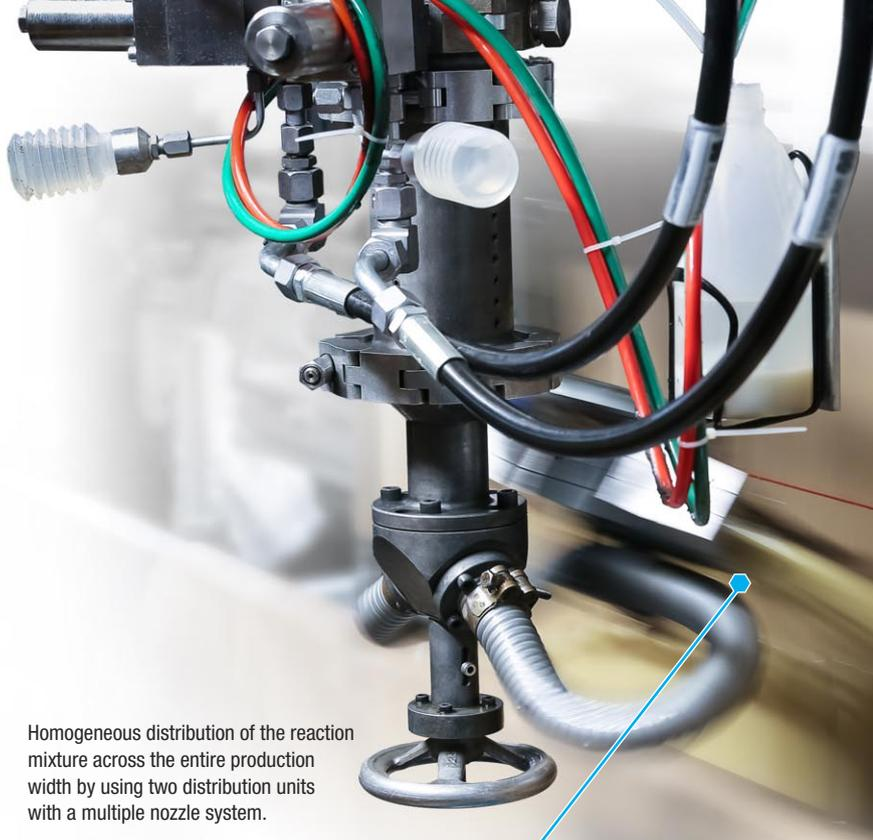
Homogeneous distribution of the reaction mixture across the entire production width by using two distribution units with a multiple nozzle system.
