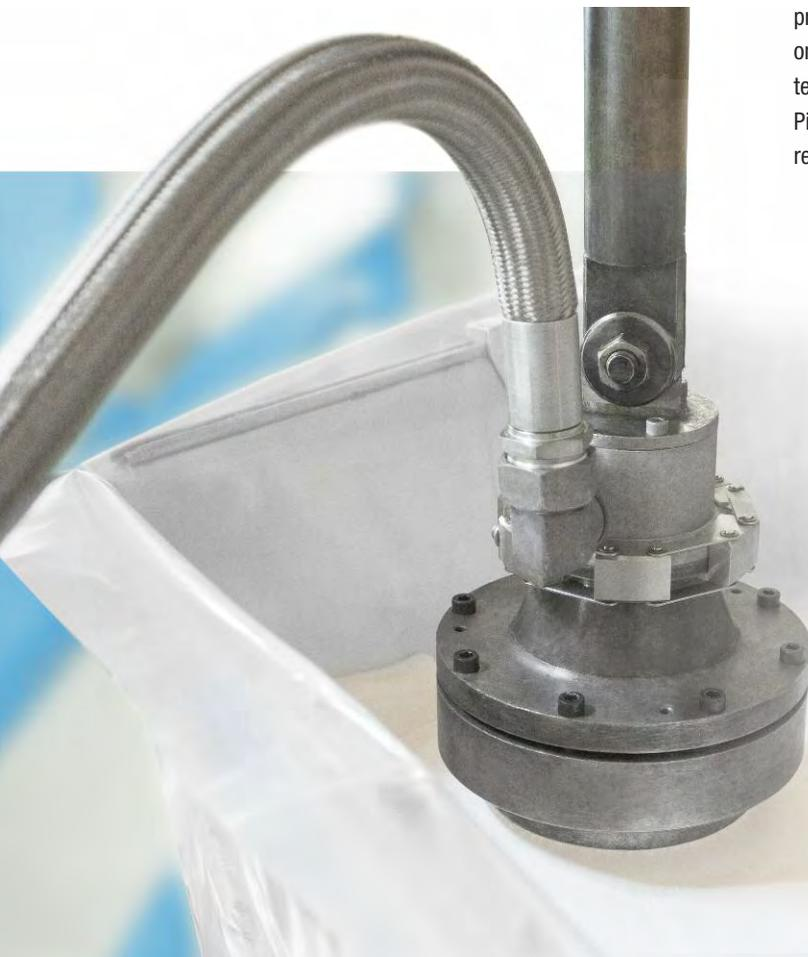
*Targeted influencing of the foam's performance characteristics or production of entirely new foam types: NOVAFLEX technology with NOVAFLEX creamer*
