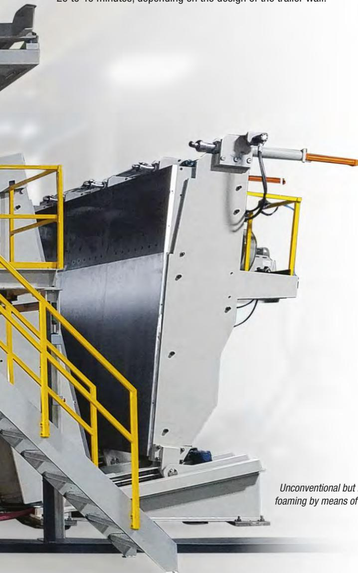
*Unconventional but highly efficient: foaming by means of the "free-rising foam method" using the A-frame double press*
