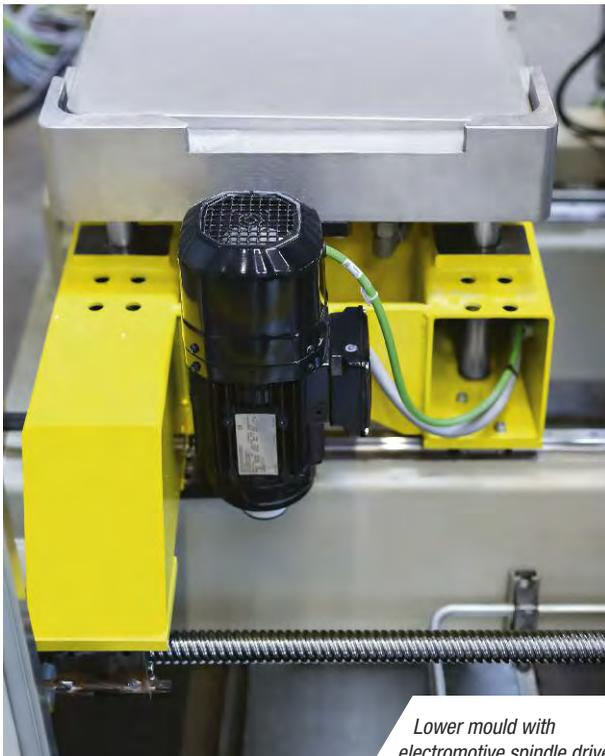
*Lower mould with electromotive spindle drive*
