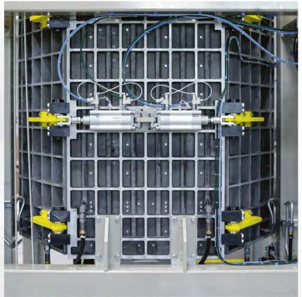
*Safe and reliable: closing and opening through pneumatic cylinder*
