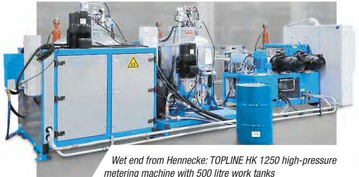
*Wet end from Hennecke: TOPLINE HK 1250 high-pressure metering machine with 500 litre work tanks*
