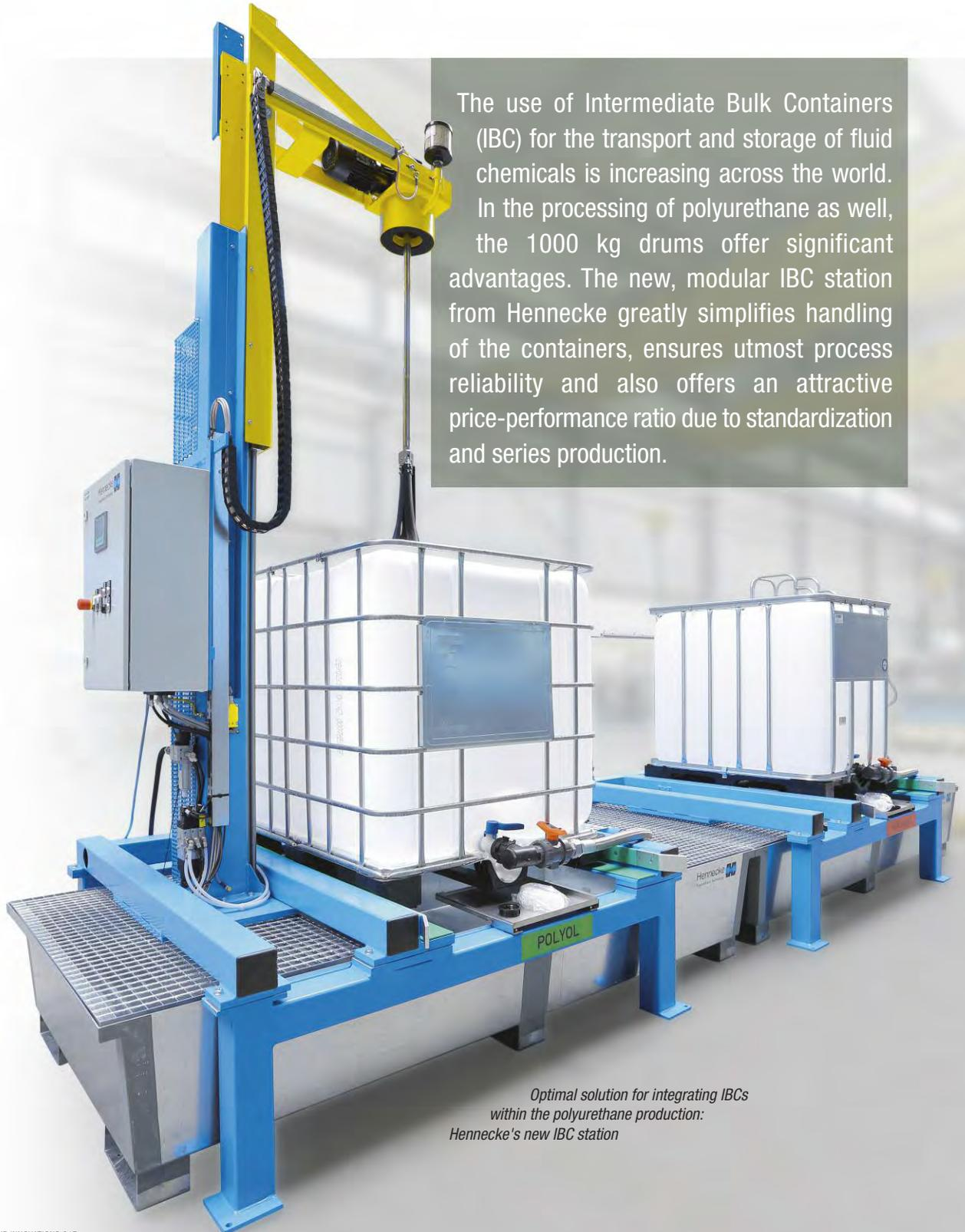
The use of Intermediate Bulk Containers (IBC) for the transport and storage of fluid chemicals is increasing across the world. In the processing of polyurethane as well, the 1000 kg drums offer significant advantages. The new, modular IBC station from Hennecke greatly simplifies handling of the containers, ensures utmost process reliability and also offers an attractive price-performance ratio due to standardization and series production.
