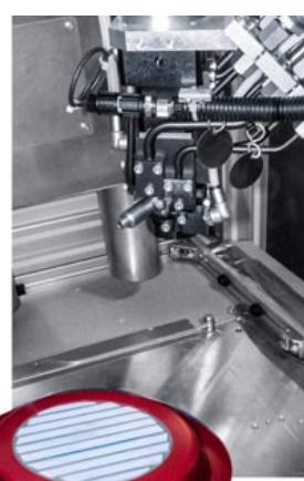
*Automated polyurea spray application for coating the filter front side*
