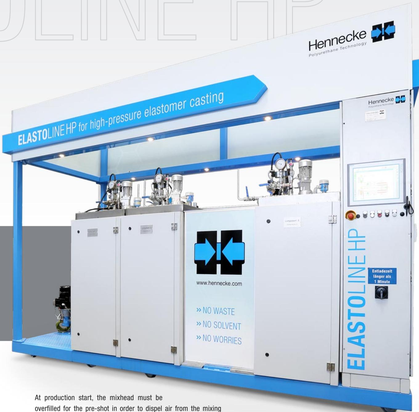
At production start, the mixhead must be overfilled for the pre-shot in order to dispel air from the mixing chamber and set the so-called stoichiometric mixture ratio despite the different viscosities. At the end of production, the mix head is completely full with material and needs to be emptied and rinsed to prevent the elastomer reaction mixture from curing in the mixer. The concluding flushing shot is different for each system.
