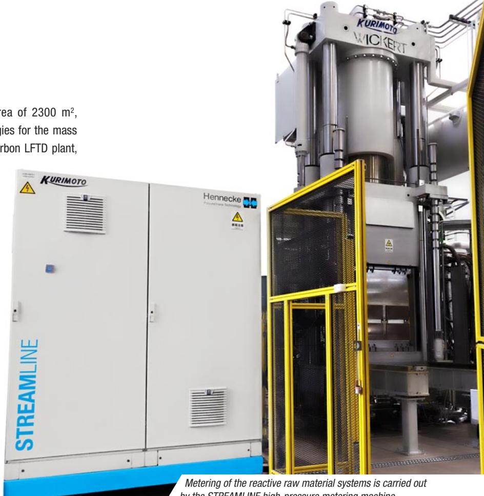
*Metering of the reactive raw material systems is carried out by the STREAMLINE high-pressure metering machine*
