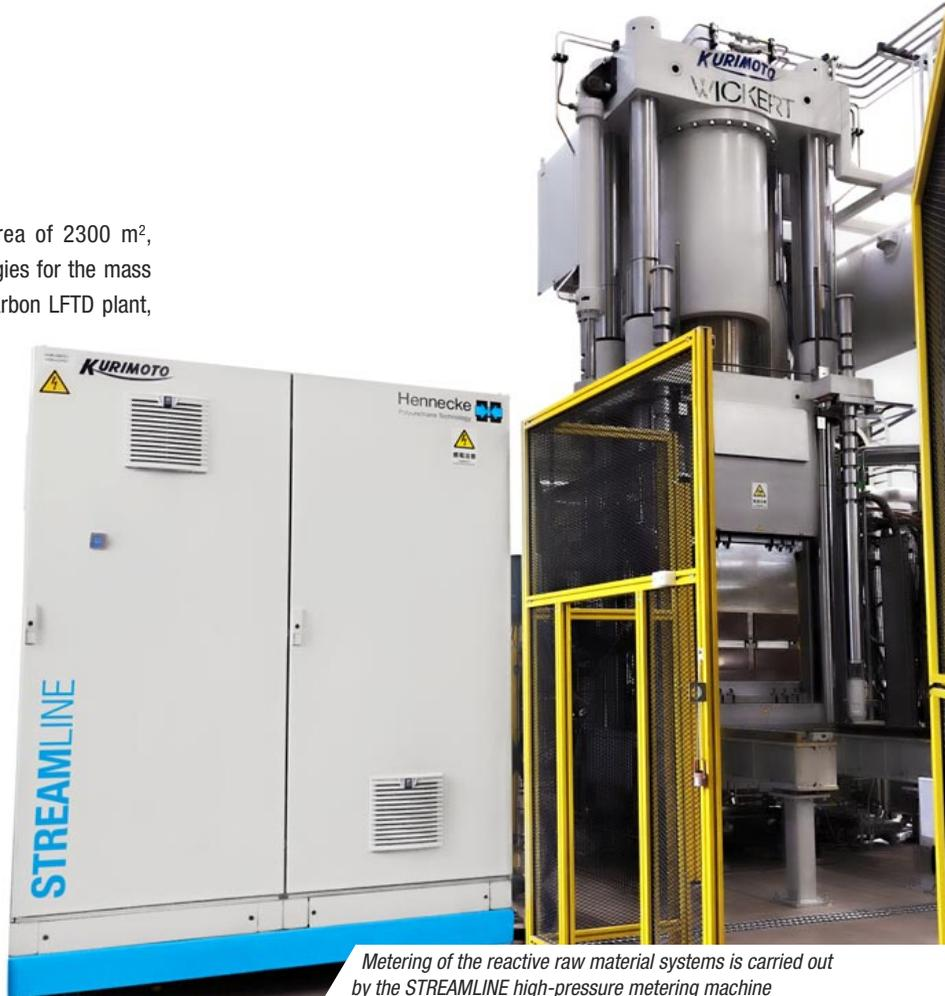
*Metering of the reactive raw material systems is carried out by the STREAMLINE high-pressure metering machine*
