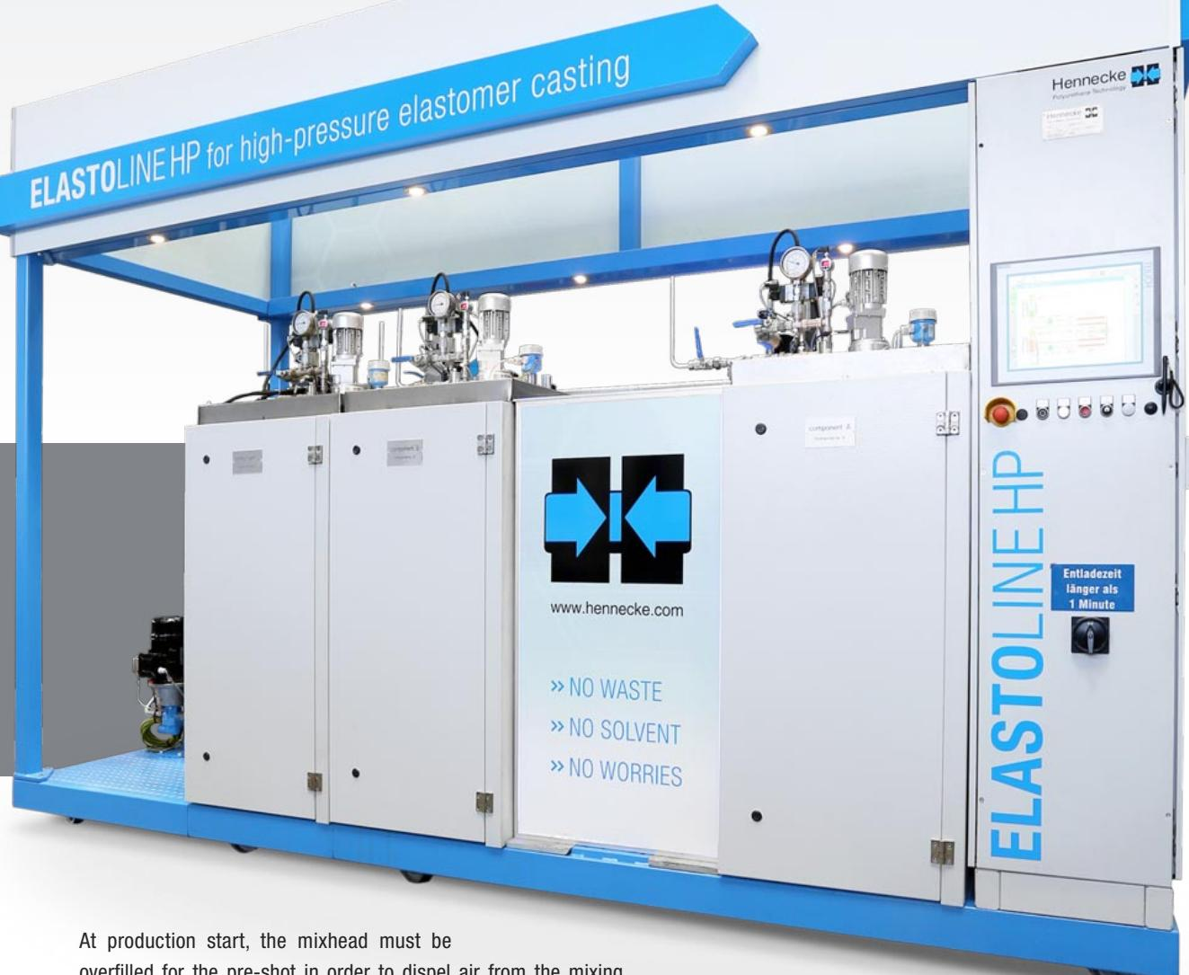
At production start, the mixhead must be overfilled for the pre-shot in order to dispel air from the mixing chamber and set the so-called stoichiometric mixture ratio despite the different viscosities. At the end of production, the mixhead is completely full with material and needs to be emptied and rinsed to prevent the elastomer reaction mixture from curing in the mixer. The concluding flushing shot is different for each system.
