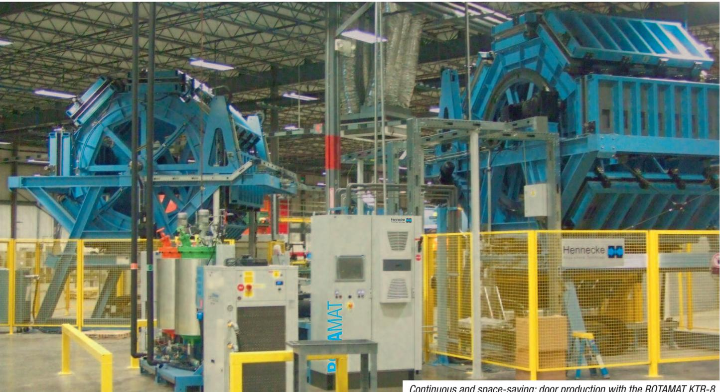
Continuous and space-saving: door production with the ROTAMAT KTR-8
