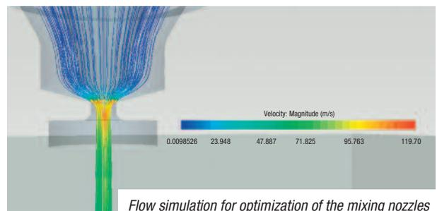
a considerably wider process window, in which a large range of products can be manufactured reliably and at the highest quality with the scrap rate also decreasing significantly. The MT series now provides users with a mixer system, which reflects the current state of the art.
