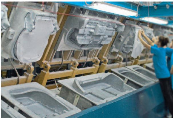
For this application, Hennecke offers its oval conveyor plant concepts with an automatic in- and outfeed station QCD (Quick-Connect-Disconnect), which allow the exchange of mould carriers during running production and at a conveyor speed of up to 15 m/min. This makes it possible to retrofit, prepare and maintain the mould carriers
