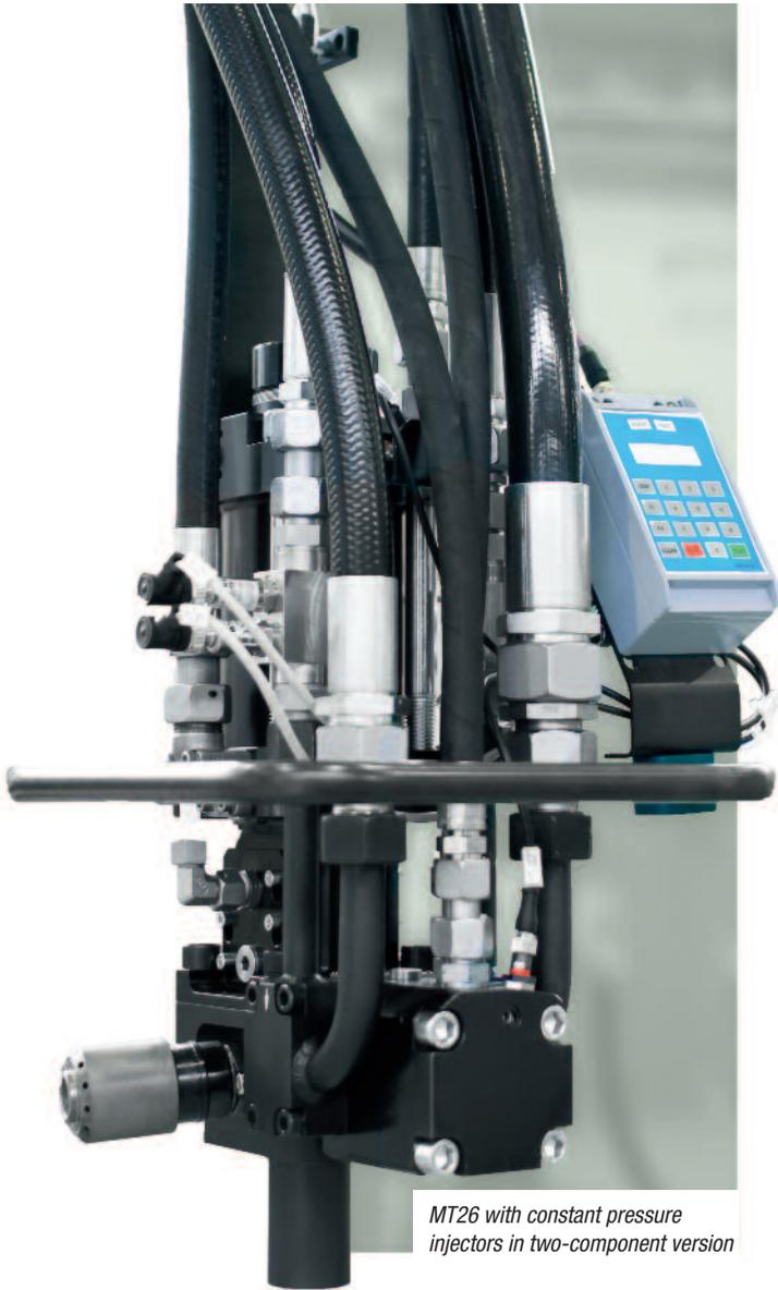
*MT26 with constant pressure injectors in two-component version*
