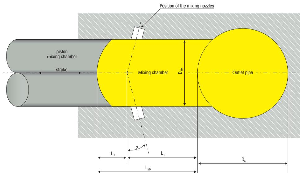
*Cross section of a high-pressure deflection mixhead*
