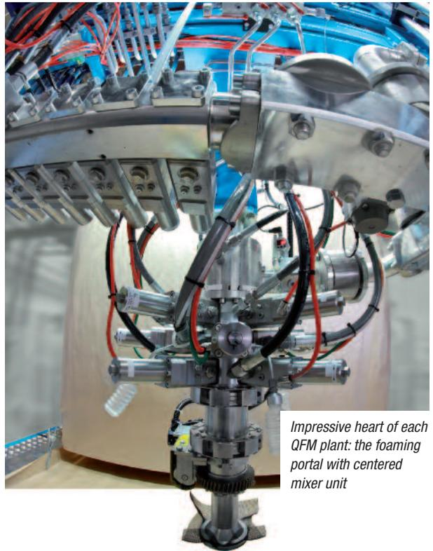
*Impressive heart of each QFM plant: the foaming portal with centered mixer unit*
