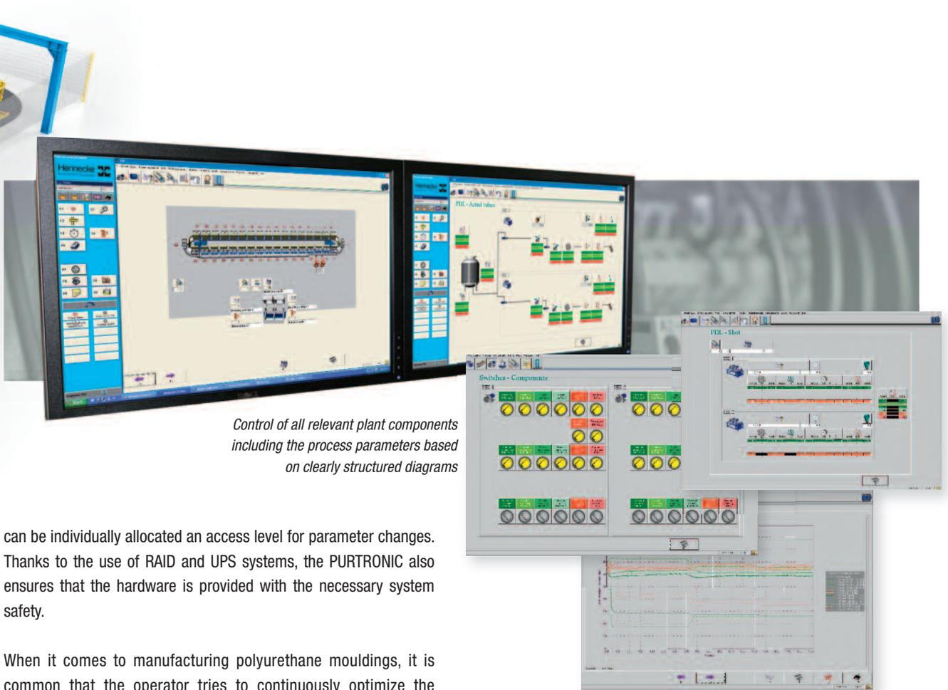
*Control of all relevant plant components including the process parameters based on clearly structured diagrams*
