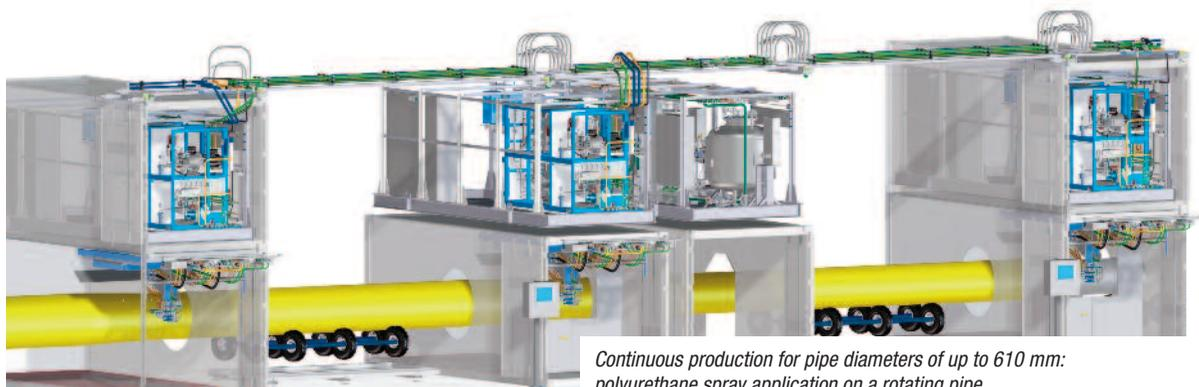
*Continuous production for pipe diameters of up to 610 mm: polyurethane spray application on a rotating pipe*
