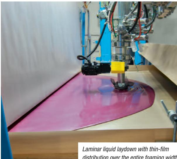
*Laminar liquid laydown with thin-film distribution over the entire foaming width*
