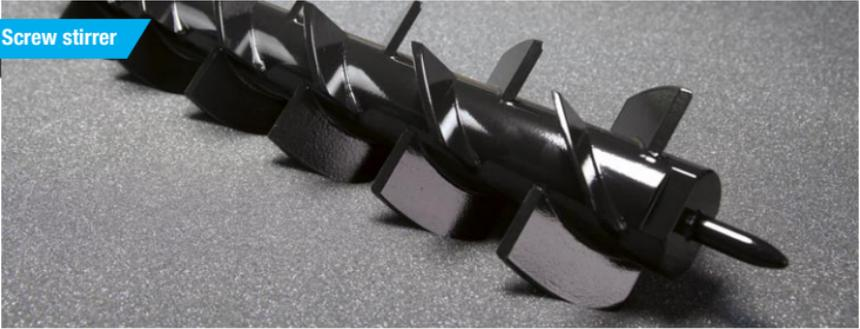
In slabstock processing, the screw stirrer is suitable for ether and ester foams that require mixing under low mixing chamber pressure at the entrance to the mixing chamber, and at the same time a high rotation speed. This stirrer therefore creates an inverted pressure profile: the formulation can thus be homogeneously mixed and particularly pressure-sensitive foams that are largely free of pinholes can be produced.
