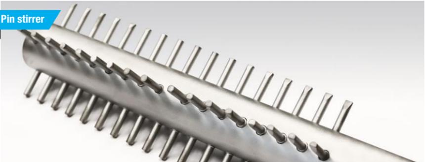
In slabstock processing, the pin stirrer is particularly suitable for ether foams that require vigorous mixing. Homogenous mixing is absolutely imperative for ether foams. When using the pin stirrer, pay attention to the increasing chamber pressure at increasing speed.
